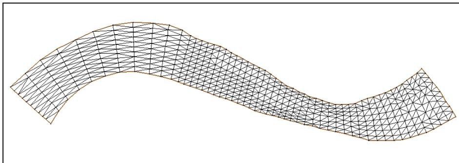
Figure 2 The poway1 mesh after deleting excess triangles
