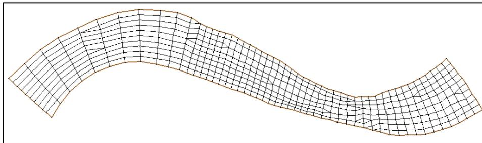
Figure 3 The poway1 mesh after merging triangles
