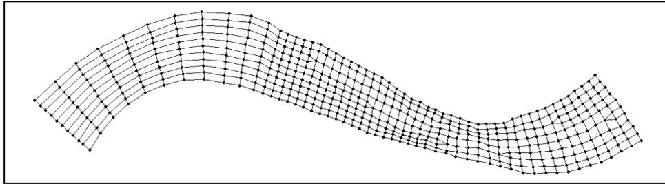
Figure 8 The finite element mesh after merging triangles
