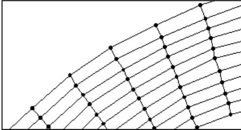
Figure 5 The mesh section after merging triangles
